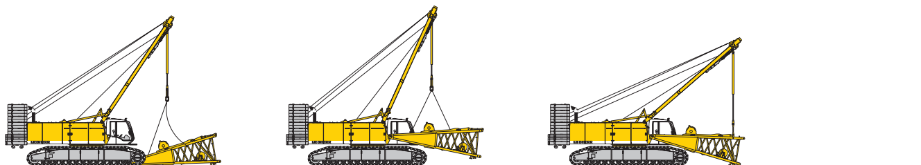
Unloading and assembly of boom foot
